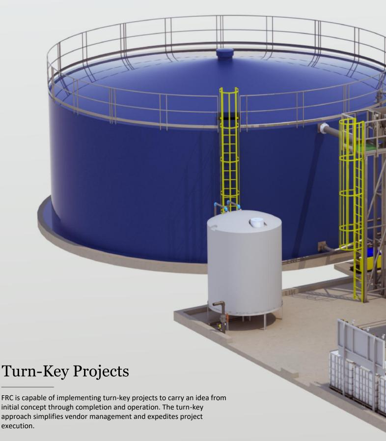
The image on this page is a 3D rendering from a turn-key system FRC installed for Trident Seafoods in Carrollton, Georgia. The process includes headworks, equalization, chemical/physical separation, biological treatment, and sludge dewatering.
