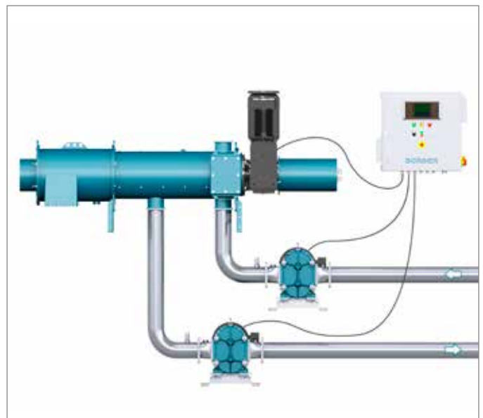
Alternatively, a liquid phase pump can convey the liquid phase to where it is used next. An intermediate container is not required.
