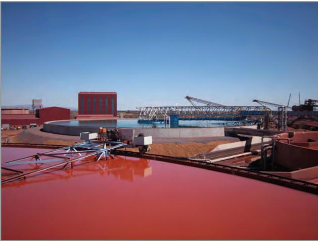
For high-tonnage / high-torque applications, a WesTech Titan™ traction thickener can be used as an ideal, economical alternative to conventional center-driven, high-rate thickeners.
