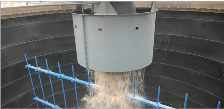
WesTech's patented EvenFlo™ Feedwell achieves peak performance with its simple two-stage design. It significantly improves the overflow clarity while using a lower flocculant dosage.
