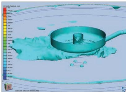
**The short-circuiting flow prematurely exits to one side from a typical tangential-feed feedwell.**
