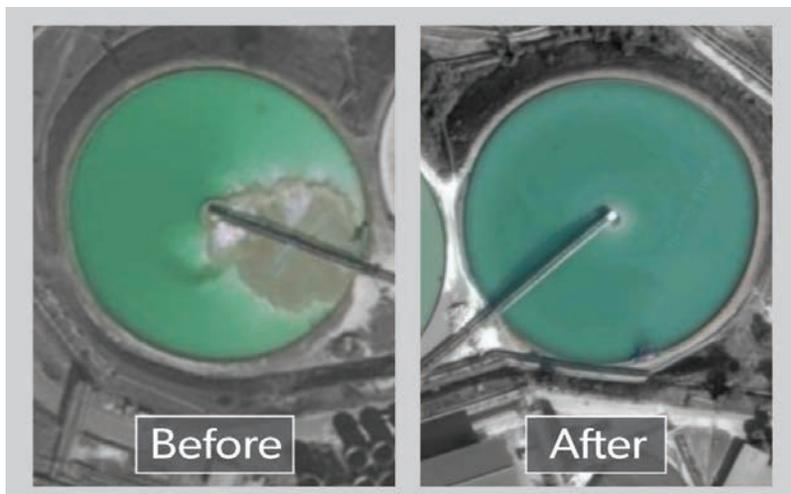
The benefits of retrofitting three 135-meter traction thickeners is shown on the left; the short-circuiting flow seen in the Before photo is corrected by retrofitting an EvenFlo Feedwell in the thickener in the After photo.
