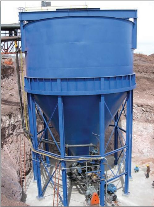
The AltaFlo™ ultra high-rate thickener is a rake-less thickener that provides mixing, flocculation and internal dilution, followed by clarification and positive sludge collection and removal, all in a single tank. The principles of dewatering have been further optimized to a new design that thickens slurries at an even higher rate than a typical high-rate thickener.
